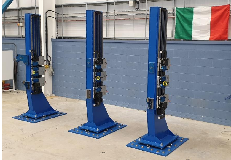
Fig. 4. VADIS Fixture Installed at Electroimpact Facility
